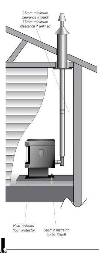
This flue kit may be used in replacement applications in rooms with stud height of 2.4m. The overall height of the flue is 3.6m. The visible flue is finished in black and the ceiling plate is white. Kit is supplied in a carton.
