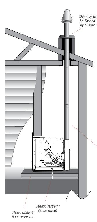
This flue kit may be used in new or existing timber chimneys. The overall height of the flue is 3.6m. Kit is supplied in a carton.
