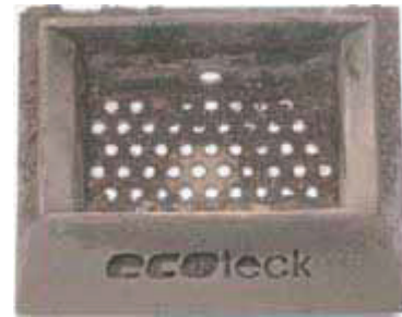
Burn pot liner needing cleaning with holes blocked by ashes
