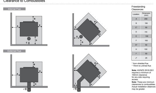
Note: The above clearance to combustibles on the flue are only applicable within the fire envelope. Clearance outside this e.g. at a ceiling / wall thimble reverts to 25mm as per ARS flue test 05/185.
