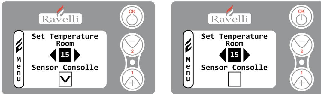
To modify the thermostat value press Key 1. Enter the Set Temperature menu and with Keys 1 and 2 set the desired room temperature at which the fire will enter Modulation Work Mode.
