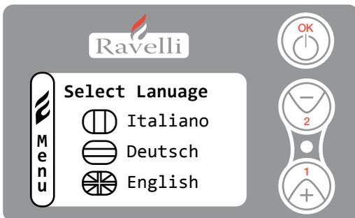
To enter, in the USER MENU press OK twice, then press key 2 five times and confirm with OK. Select your desired language using keys 1 and 2. Save your selection by pressing OK. To return to the main screen press keys 1 and 2 at the same time.
