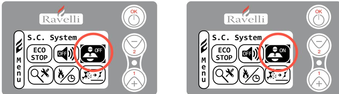
To enter, in the USER MENU press the OK key twice then to enter the SELF CONTROL SYSTEM mode press key 2 eight times and confirm with OK. Enable or disable the function by using the OK key. To return to the main screen press keys 1 and 2 at the same time.
