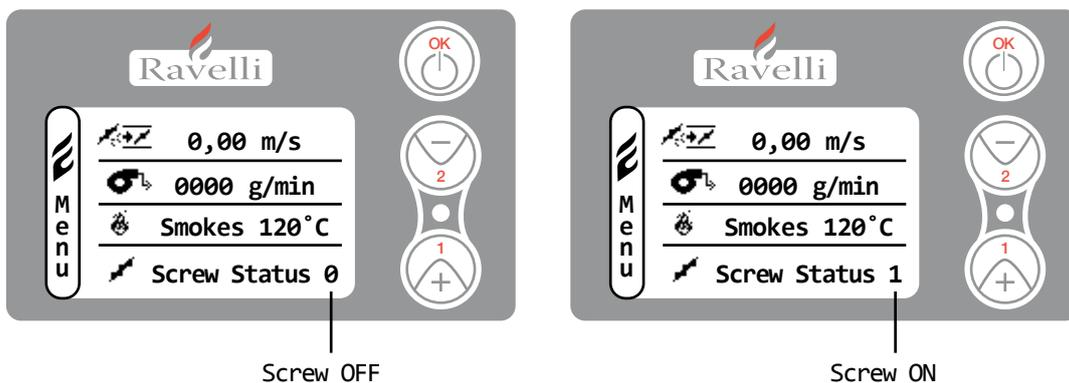
To return to the main screen press keys 1 and 2 at the same time. Repeat the operation several times until you see the pellets fall into the firepot. It is possible to do this operation only if the stove is in FINAL CLEANING phase or OFF.
