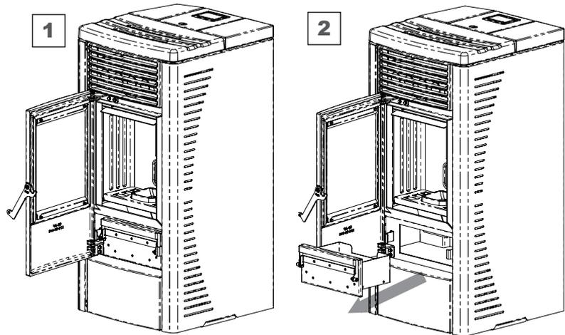
**HOW TO REMOVE THE FLAME TRAP:**
