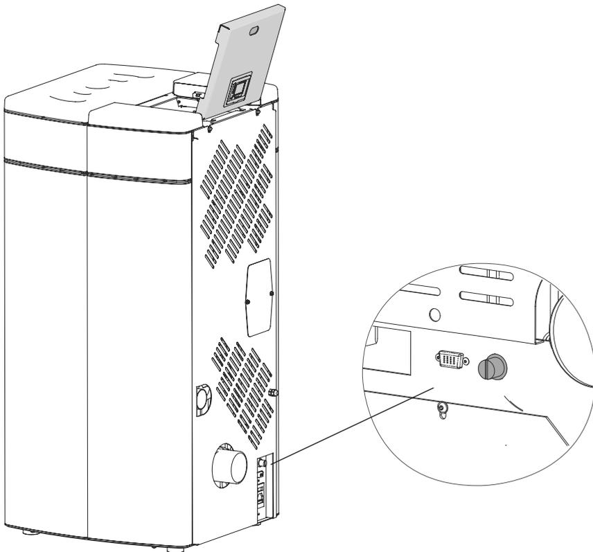
Unscrew the protection cap and press the button to reset the thermostat alarm.
