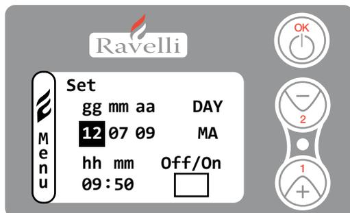
To enter, in the USER MENU press the OK key twice, then press key 2 three times and confirm with OK. To modify settings use keys 1 and 2 and by pressing OK you can confirm data and move to the next area. By activating the ON/OFF box you enable the CHRONOTHERMOSTAT function (see 6.5.5 on page 17). To return to the main screen press keys 1 and 2 at the same time.
