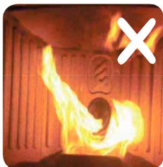
The combustion is **NOT CORRECT**, the flame is weak and a lot of unburned pellet wood into the firepot. Check first that the ash pan is properly closed. Then adjust set pellet/air increasing the air percentage (from 0 up to +5); in the event this is not enough, increase the loading quantity of the pellet (from 0 up to -5) to reach the flame condition shown in picture 3.
