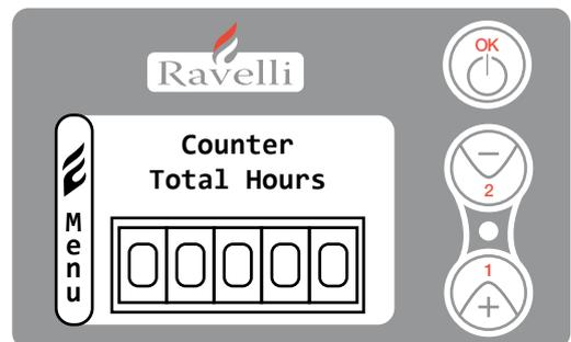
To enter, in the USER MENU press the OK Key twice then to enter the VIEW WORKING HOURS menu, press key 2 ten times. By confirming with OK you can see the working hours of the stove. To scroll through the different counters (total or partial hours and number of ignitions) use key 1 and 2. To return to the main screen press keys 1 and 2 at the same time.
