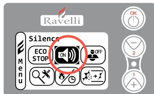
SILENCE mode reduces the noise level of the fan by reducing the fan speed at all five heat levels. You
