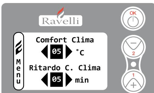
eg room temperature set at 21° with Comfort Clima value set at 5. The pellet fire will switch off when 21°C is reached and will switch back on when the room temperature is 18°C (21°C – 2 – 0,5 = 18°C). The following strings will appear in sequence on the display:
