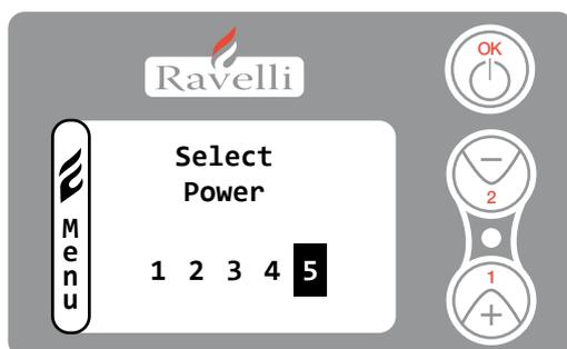
To modify the working power press key 2 to enter in the dedicated menu and with keys 1 and 2 to set the power you desire from 1 to 5 and confirm with key OK. Increasing the power also increases pellet consumption and the speed of the fan. It is not possible to modify the set power during the phase of MODULATION WORK.
