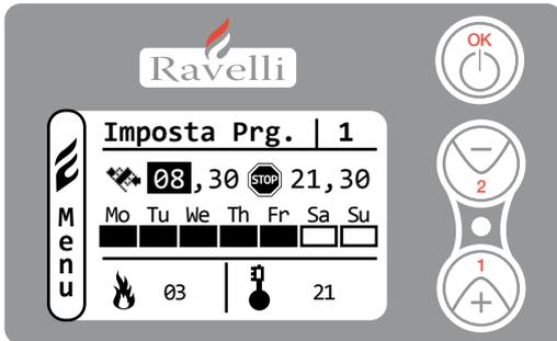
Using the OK key, move to the time setting area, and set the ‘Switch On’ time using keys 1 and 2.
