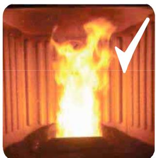
The combustion **IS CORRECT**, full flame yellow/white and minimum quantity of pellet in the firepot.
