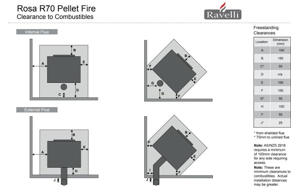
Note: The above clearance to combustibles on the flue are only applicable within the fire envelope. Clearance outside this e.g. at a ceiling / wall thimble reverts to 25mm as per ARS flue test 05/1185.
