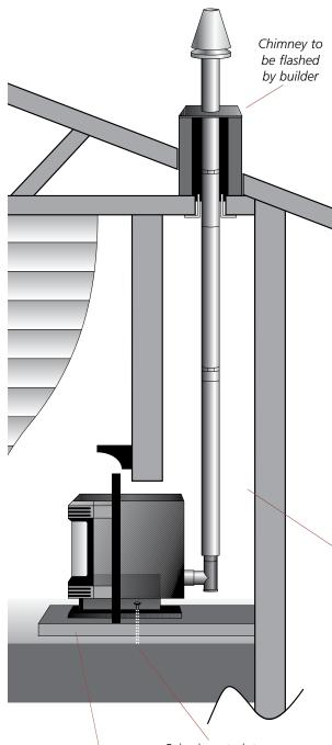
Heat-resistant floor protector Seismic restraint (to be fitted) This flue kit may be used in new or existing timber chimneys. The overall height of the flue is 3.6m. Kit is supplied in a carton.
