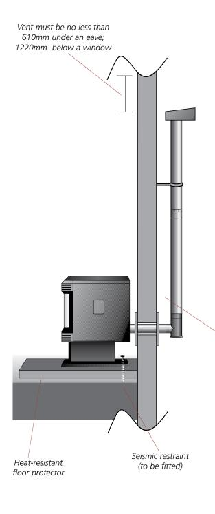
This flue kit may be used in new and replacement applications with the flue penetrating the wall behind the fire, running vertically up an outside wall and the flue venting horizontally from the vent. This must not be under a soffit. The overall height of the flue is 2.7m. All visible flue has a galvanised finish, and can be powdercoated on request. Kit is supplied in a carton.
