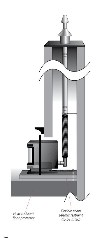
This flue kit may be used in replacement applications in masonry chimneys. The overall height of the flue is 5.5m. Kit is supplied in two cartons.
