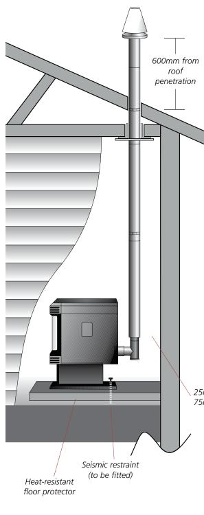
This flue kit may be used in new and replacement applications in rooms with stud height of 2.4m. The overall height of the flue is 3.6m. The visible flue is finished in black and the ceiling plate is white. The support angles for securing the liner to the ceiling are not shown. Kit is supplied in a carton.
