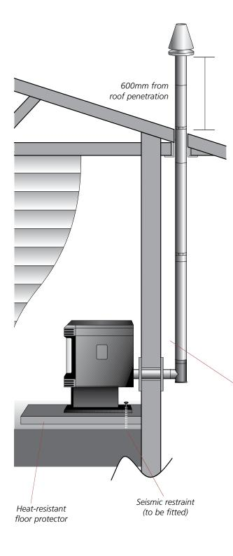
This flue kit may be used in new and replacement applications with the flue penetrating the wall behind the fire, running vertically up an outside wall and penetrating the soffit. The overall height of the flue is 3.6m. All visible flue has a galvanised finish, and can be powdercoated on request. Kit is supplied in a carton.
