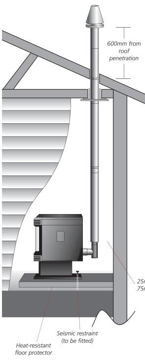
This flue kit may be used in new and replacement applications in rooms with stud height of 2.4m. The overall height of the flue is 3.6m. The visible flue is finished in black and the ceiling plate is white. The support angles for securing the liner to the ceiling are not shown. Kit is supplied in a carton.
