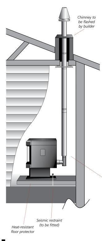
This flue kit may be used in new or existing timber chimneys. The overall height of the flue is 3.6m. The visible flue is finished in black and the ceiling plate is white. The support angles for securing the liner to the ceiling are not shown. Kit is supplied in a carton.
