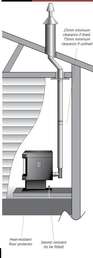
This flue kit may be used in new and replacement applications where the roof opening is off-centre to the internal flue, in rooms with stud height of 2.4m. The overall height of the flue is 3.6m. The visible flue is finished in black and the offset ceiling plate is white. Kit is supplied in a carton.
