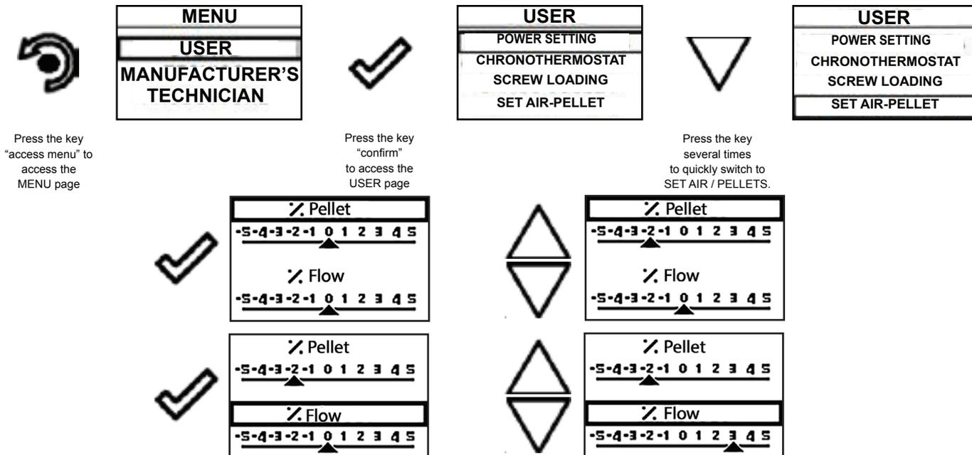
As per the above example, you have set a percentage of -2 for PELLETS and +3 for the FLOW, an indication that a setting like this is a consequence of the fact that the oxygen needed for combustion is insufficient and pellet size is smaller than the average size of 2 cm.
