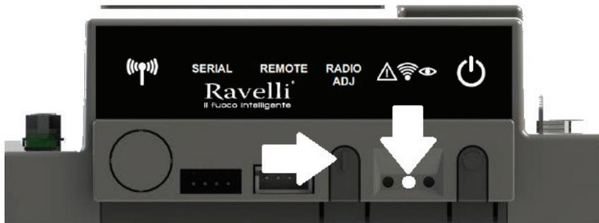
The flashing yellow LED indicates that the circuit board is waiting to receive the signal from the handheld set.
