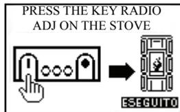
Hold down for a few seconds the button of radio communication (RADIO ADJ) of the PCB, located on the back of the stove, to initialize the device.
