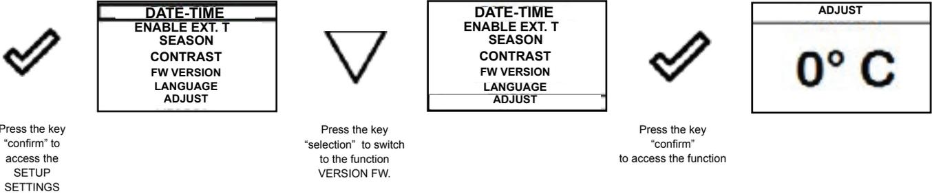
Use the UP/DOWN keys to change the value read by the room temperature probe installed inside the handheld set, with respect to a reference value. The value can vary from -10°C to 10°C. The standard value is 0°C.
