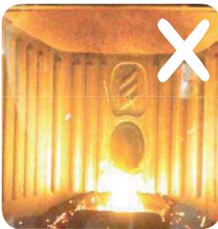
**INCORRECT** combustion - the flame is weak and there are a lot of unburned pellets in the firepot. Check first that the ash pan is properly closed. Then adjust set pellet/air increasing the air percentage (from 0 up to +5). If this doesn't work, try increasing the loading quantity of the pellet (from 0 up to -5) to reach the flame condition shown in picture 3.
