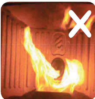
The combustion is **NOT CORRECT**, the flame is weak and a lot of unburned pellet wood in the firepot. Check first that the ash pan is properly closed. Then adjust set pellet/air increasing the air percentage (from 0 up to +5); in the event this is not enough, increase the loading quantity of the pellet (from 0 up to -5) to reach the flame condition shown in picture 3.
