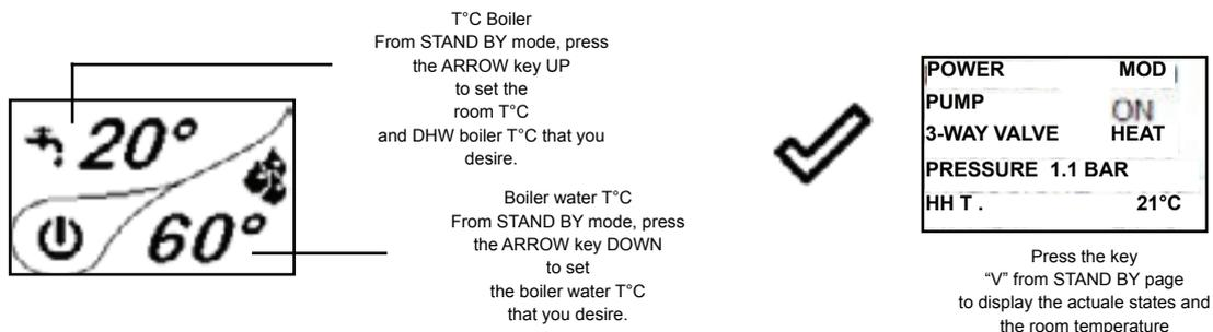
The operation is the same as for the basic layout except for the fact that in this layout, the boiler exchanges heat directly in the boiler (priority); when the temperature set is reached, the 3-way valve changes its position and the boiler starts exchanging heat within the heating circuit. From this moment, the stove is controlled by the radio handheld unit for controlling the room temperature or via H2 setting (see the operation with layout 0 to find the data on modulation, eco stop etc.).
