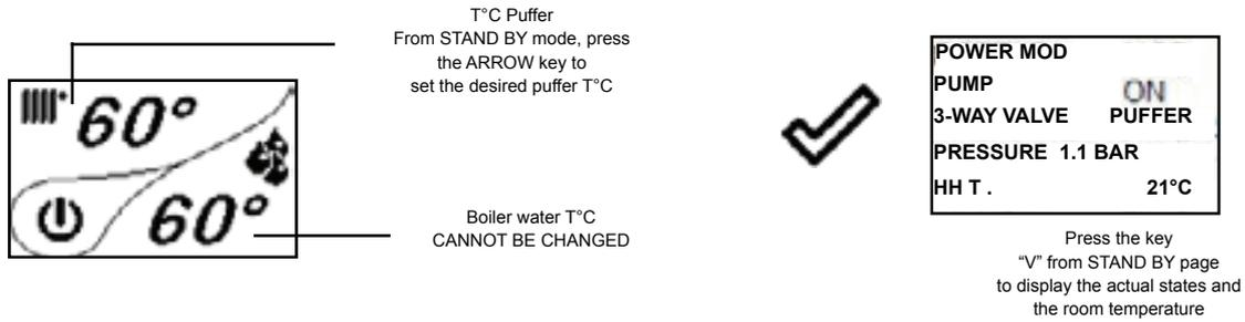
The operation is the same as for the basic layout except for the fact that in this layout, the boiler exchanges heat directly in the puffer; when the temperature set is reached, the stove switches to ECO STOP mode and then restarts if the temperature drops below a restart value (set by the installer upon testing).
