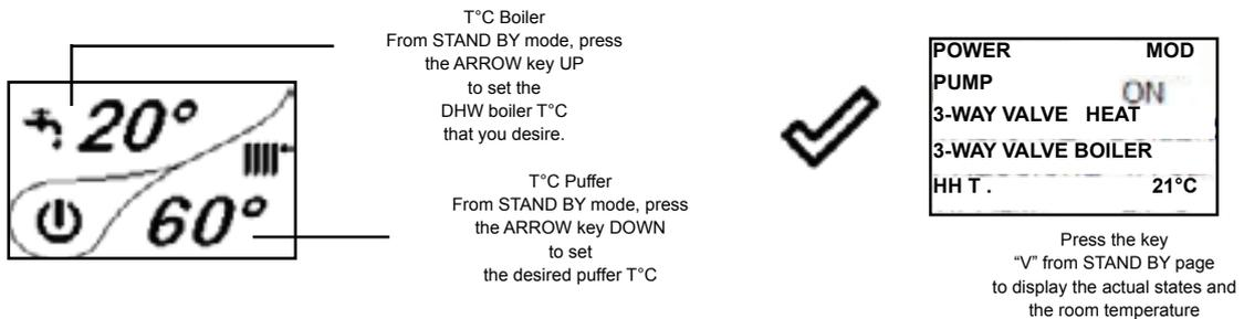
The operation is the same as for the basic layout except for the fact that in this layout, the boiler exchanges heat directly in the boiler (priority); when the temperature set is reached, the 3-way valve changes its position and the boiler starts exchanging heat within the puffer. When the set temperature is reached, the stove enters in ECO STOP mode; it restarts if the temperature drops below a restart value (set by the installer upon testing).
