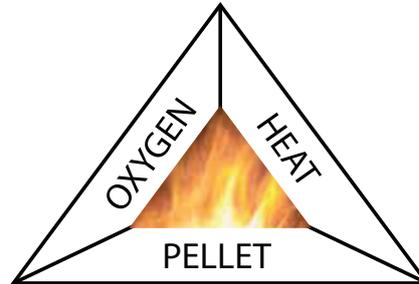
To achieve combustion, the combustible and the carburant must be available in the correct proportions.
