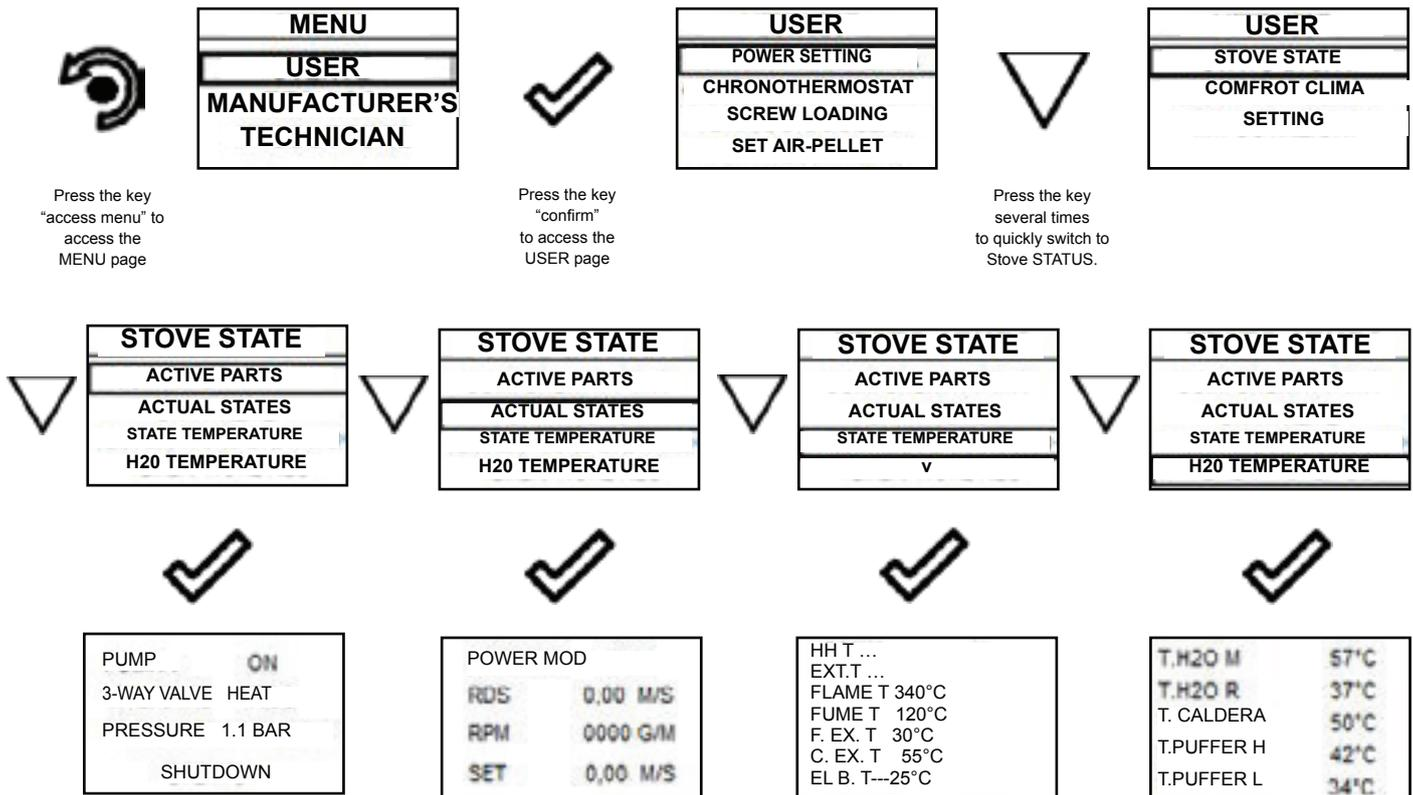
In this mode you can check the proper operation of the most important parameters of the appliance. Here is a list of real data of the stove useful for service during inspection.
