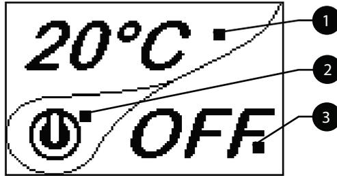
**i** After 5 minutes of inactivity, the display of the handheld set turns dark, switching to "SLEEP" mode, while maintaining the radio connection with the stove. By pressing the key ON/OFF, the display becomes active again.
