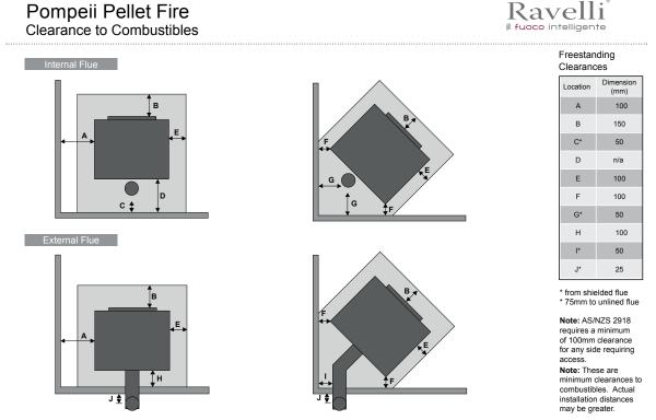
Note: The above clearance to combustibles on the flue are only applicable within the fire envelope. Clearance outside this e.g.at a ceiling / wall thimble reverts to 25mm as per ARS flue test 05/1185.
